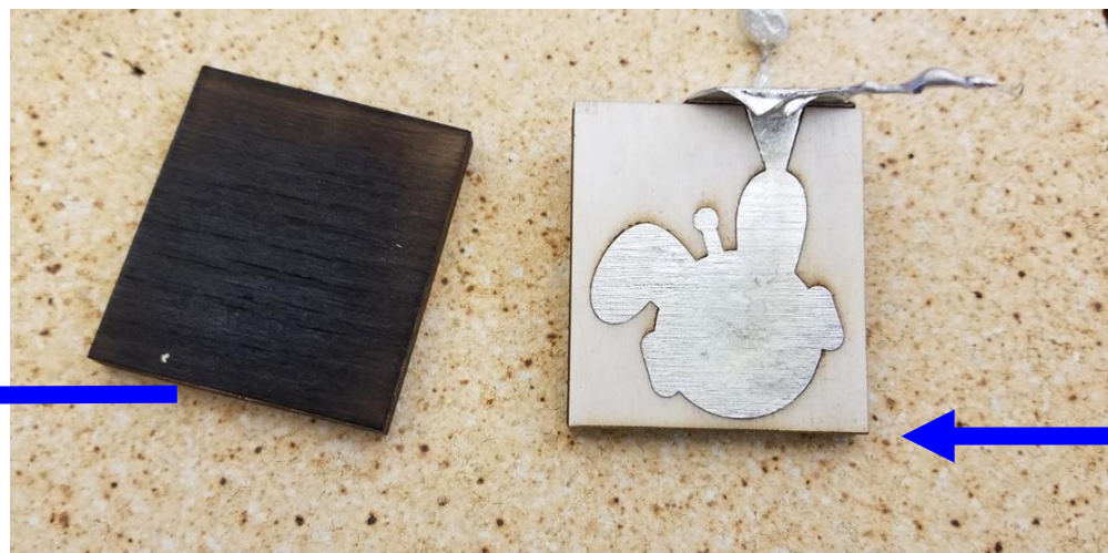
Pour pewter in mould and take apart mould once cooled
